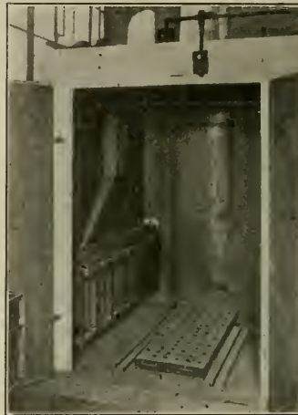
BAKING OVEN. HEATERS ON SIDE WALLS. VENTILATION AT SIDES AND ON FLOOR.
